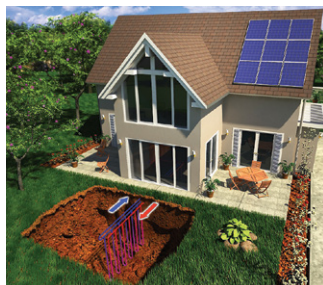
Vertical Ground Loop System
