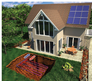
Horizontal Ground Loop System
