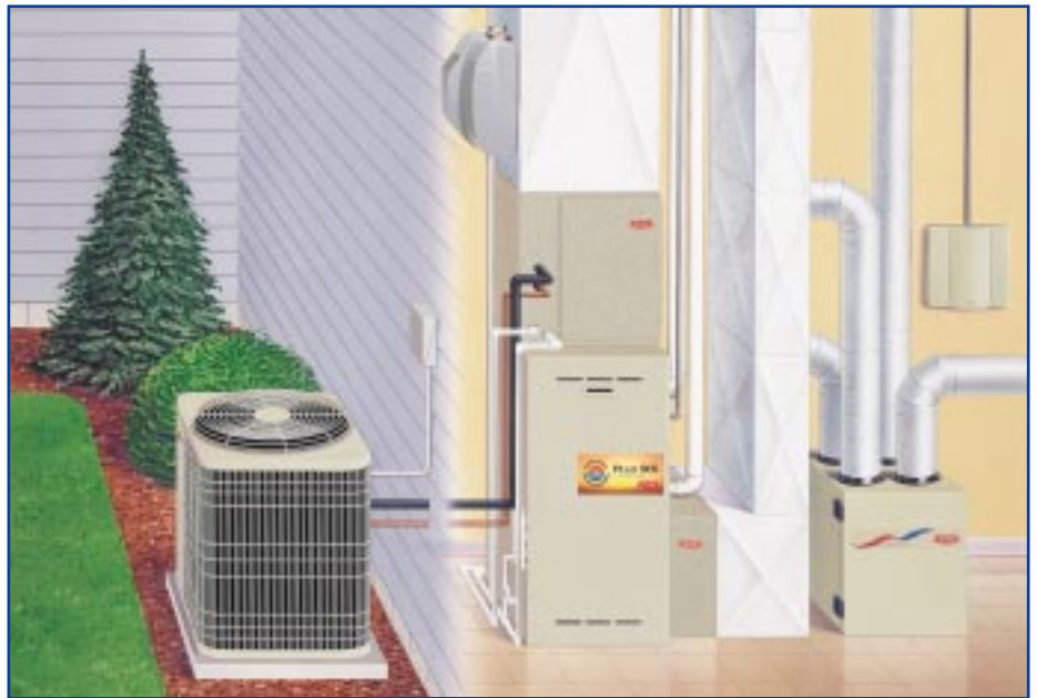
Central Air Conditioner and Gas Furnace System
