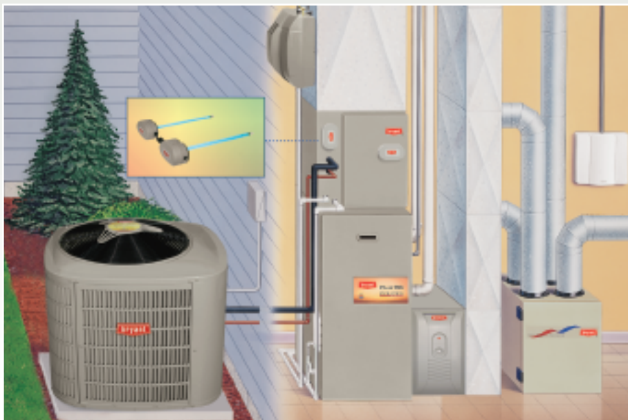
Air Conditioner and Gas Furnace System
